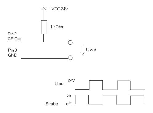
The pin numbers can be different at the camera model you use. The "U out" to "Strobe on off" relation depends on strobe polarity, if available on your camera.
