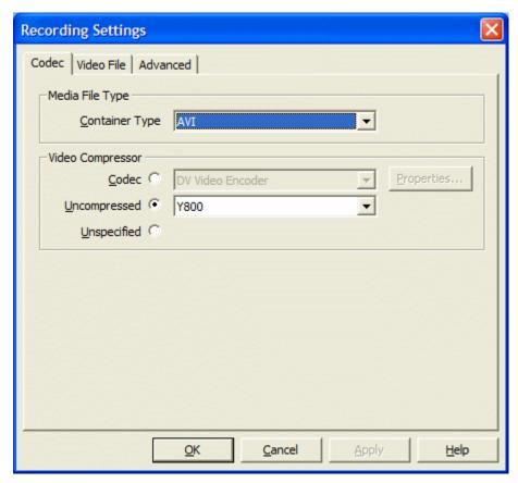
Check the radio button next to Uncompressed and select Y800 from the selection list. You can also specify further properties, such as the filename and number of frames to be captured.
