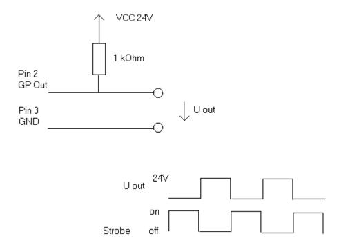
The pin numbers can be different at the camera model you use. The "U out" to "Strobe on off" relation depends on strobe polarity, if available on your camera.
