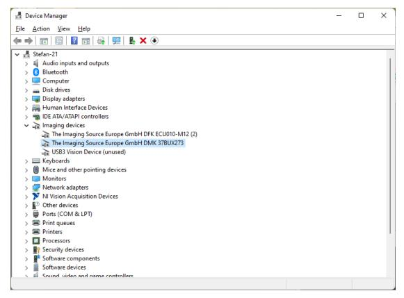
The camera is usually in "Imaging Devices", sometimes in "Cameras" section. If the driver is not installed, the camera name is shown only. Select your camera and right click on it. From the now showing context menu select "Update driver".
